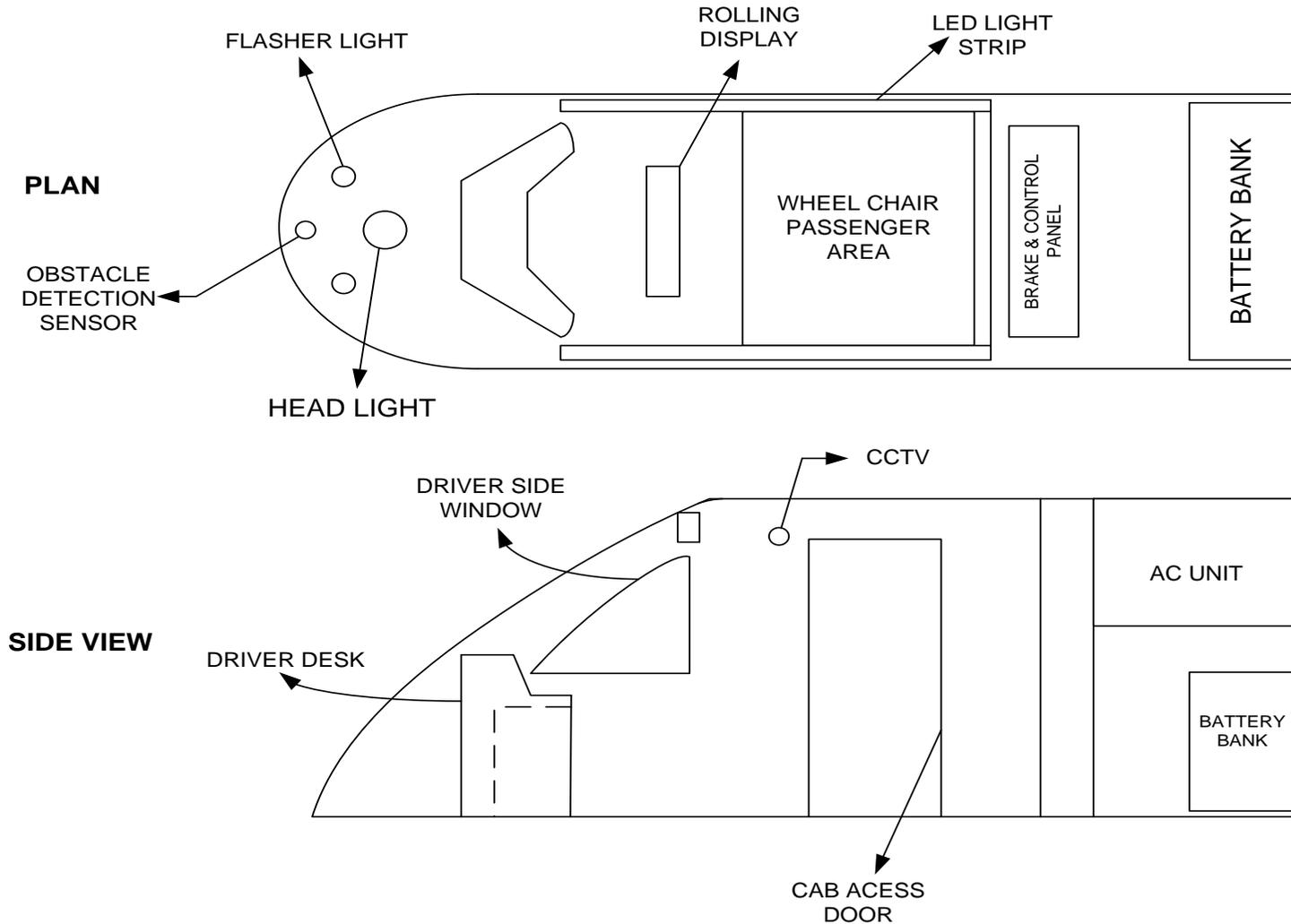
**Figure 3: DMC Equipment Location**
