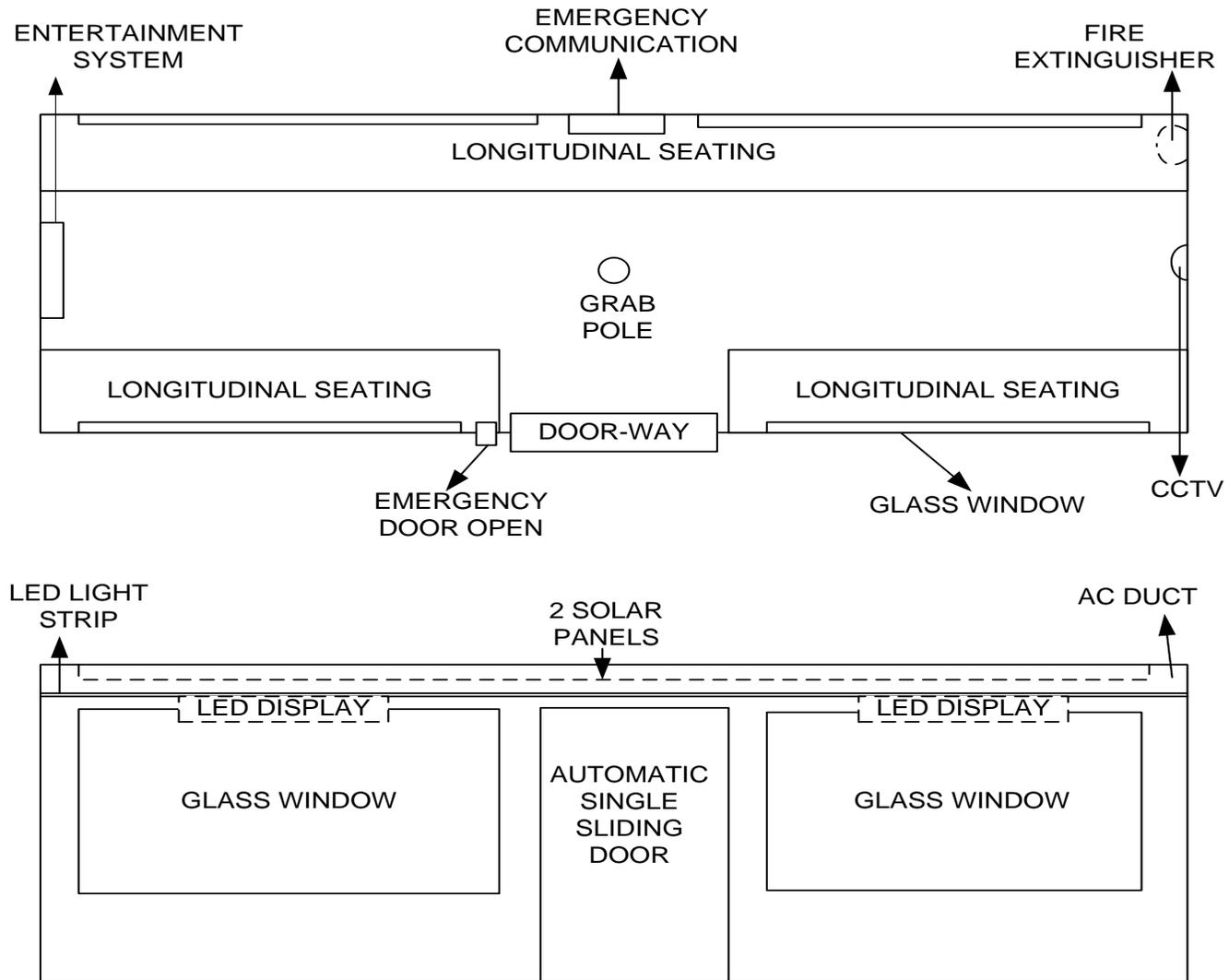
Figure 4: Layout of Equipment in Trailer Car
