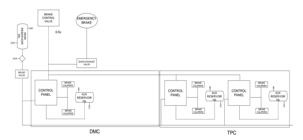
Figure 13: Pneumatic Control Circuit
