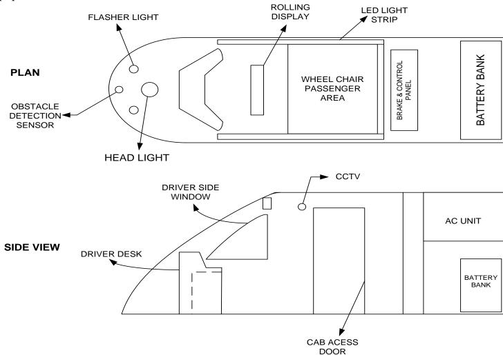
Figure 3: DMC Equipment Location
