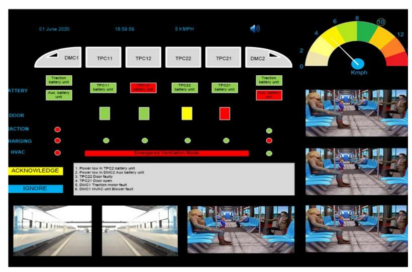
Figure 8: TCMS HMI Layout
