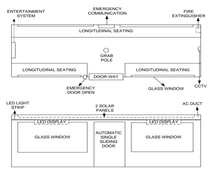
Figure 4: Layout of Equipment in Trailer Car
