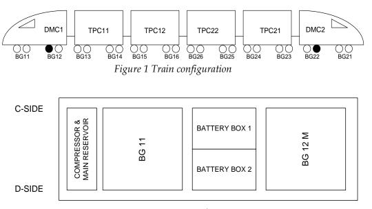
Figure 1: DMC Configuration
