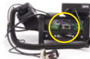
2. Undo antenna cable and D-sub connector.
