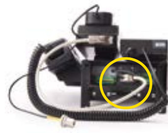
4. Connect the D-sub connector and the antenna cable.
