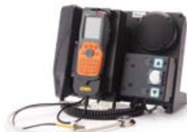
3. Mount the bayonet bracket for the Cradle kit SED.
