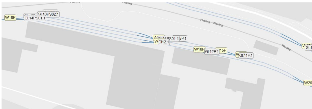
Figure 1. example of a basic digital track model (BTDM)
