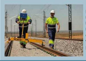
Inspired by our professionalism and customer-oriented values we developed the tCat as an internal R&D project a device to measure the geometrical parameters of the contact wire +10 years ago, which we've been consistently using in our own projects since then.
