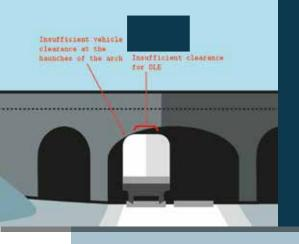
Gauge, the available space between the track, the train, the OCS and other structures such as bridges or tunnels is a critical design parameter that must also be monitored during installation, acceptance tests and line operations.
